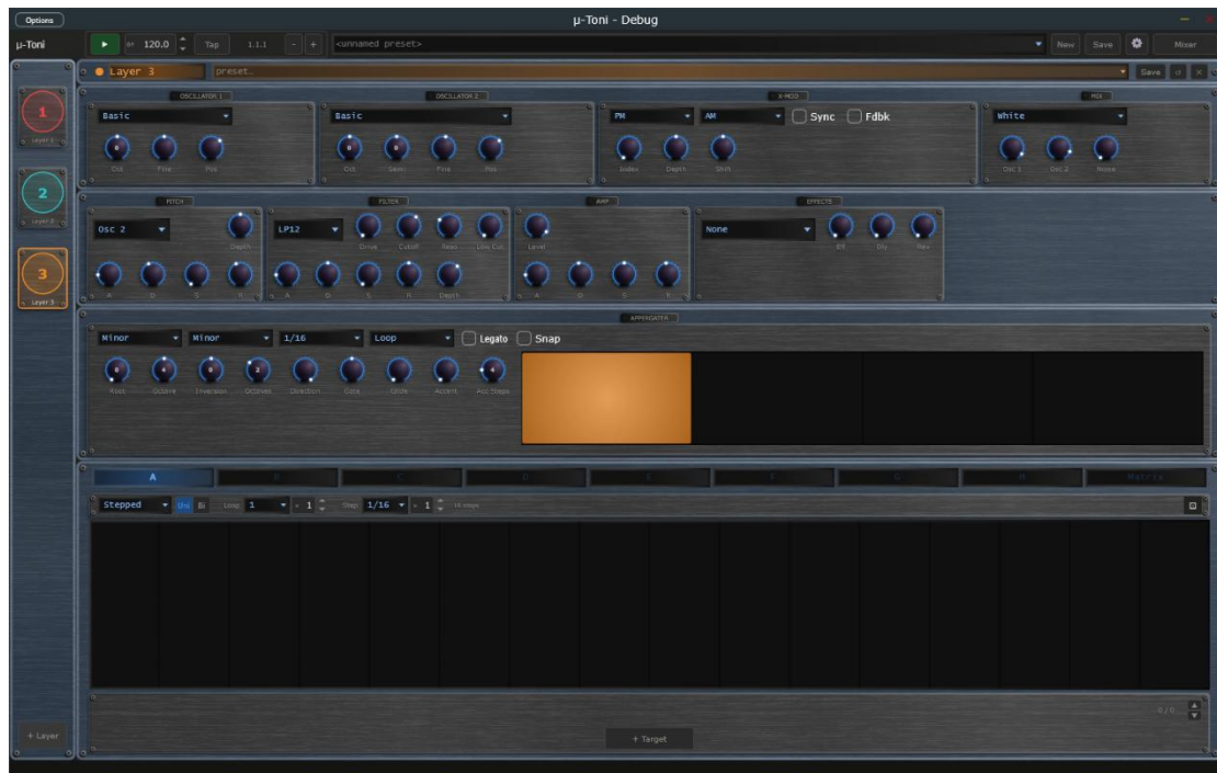
The mu-Toni window: transport bar, layer sidebar, sound sections and the Arpeggiator.
